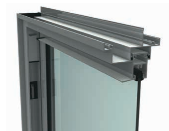
Easy take out clips on side jambs for removal of sash.
